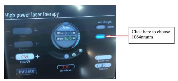
● If you need to output 980nm+1064nm at the same time, click the buttons of 980nm and 1064nm at the same time. At this time, the 980nm laser and the 1064nm laser are simultaneously out put.
