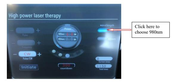
• If you need to use the 1064nm laser, you can click the switch button 1064nm laser. The output laser wave is 1064nm laser.
